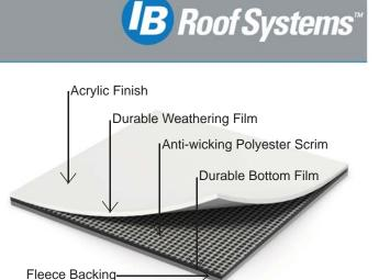
Solar Reflectance / Thermal Emittance / Calculated SRI Values Thermal **SRI Value SRI Value** Membrane Solar LRV Reflectance Emittance Initial 3-Year Aged Color White 0.870 0.88 110 91 94.3
