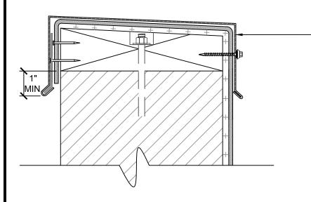
METAL COPING WITH CONTINUOUS CLEAT (SPECIFIED BY OTHERS) SECURE COPING AND NAILER TO MEET PROJECT WIND LOADS AND ES-1 AS REQUIRED
