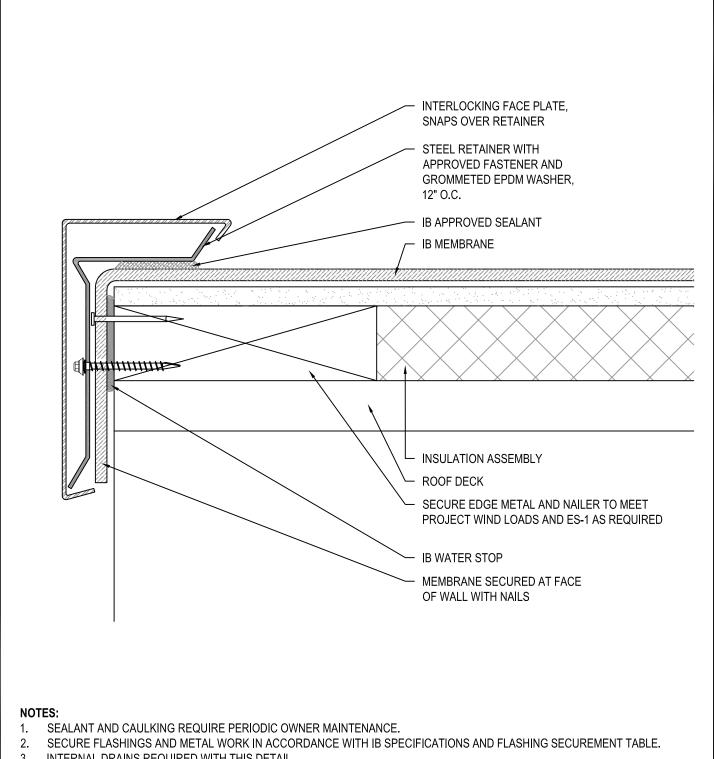
INTERNAL DRAINS REQUIRED WITH THIS DETAIL.
