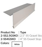
Fabricated with a durable 45 mil non-reinforced IB PVC film with acrylic finish. laminated to 24 gauge, 304 Stainless Steel sheet metal. It is formed into a gravel stop edge profile with 3/4" rise and a hemmed kick-out at the bottom to provide a corrosion resistant, heat-weldable perimeter roof edge termination.
