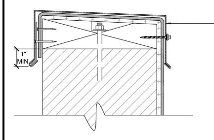
METAL COPING WITH CONTINUOUS CLEAT (SPECIFIED BY OTHERS) SECURE COPING AND NAILER TO MEET PROJECT WIND LOADS AND ES-1 AS REQUIRED
