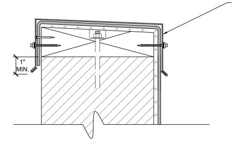
METAL COPING (SPECIFIED BY OTHERS) SECURE COPING AND NAILER TO MEET PROJECT WIND LOADS AS REQUIRED
